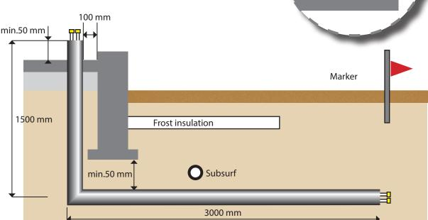
Outside the house, there must be half a metre of work space at the end of the connecting pipe for welding and special work. Subsurface drains, rain pipes and electrical cables must not be installed in the vicinity of the end of the pipe. The plastic protective cover of the vertical section of the connecting pipe must reach above the final floor casting by about 5–10 cm.
